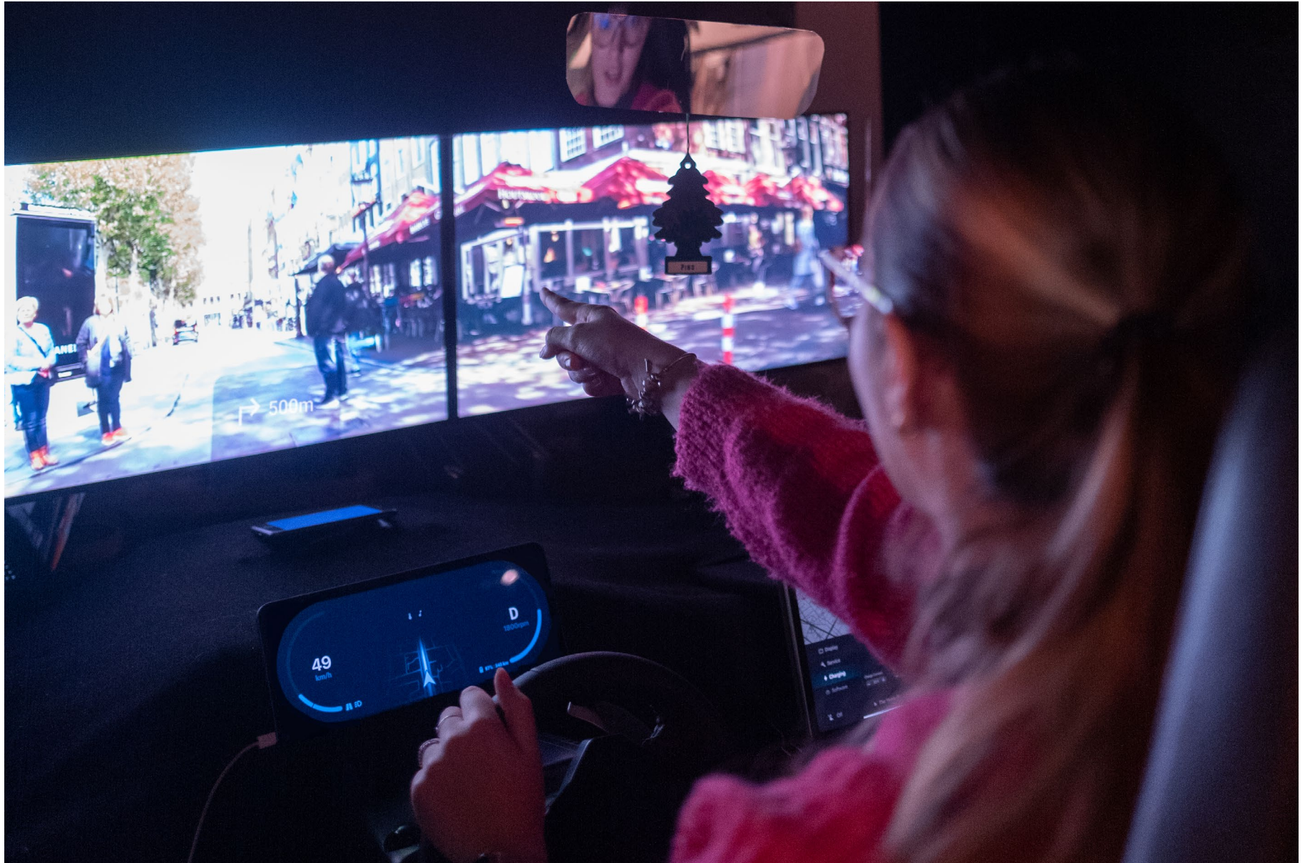
full-scale prototype during a showcase: HUD, cluster screen, center sonsole, and physical slider
