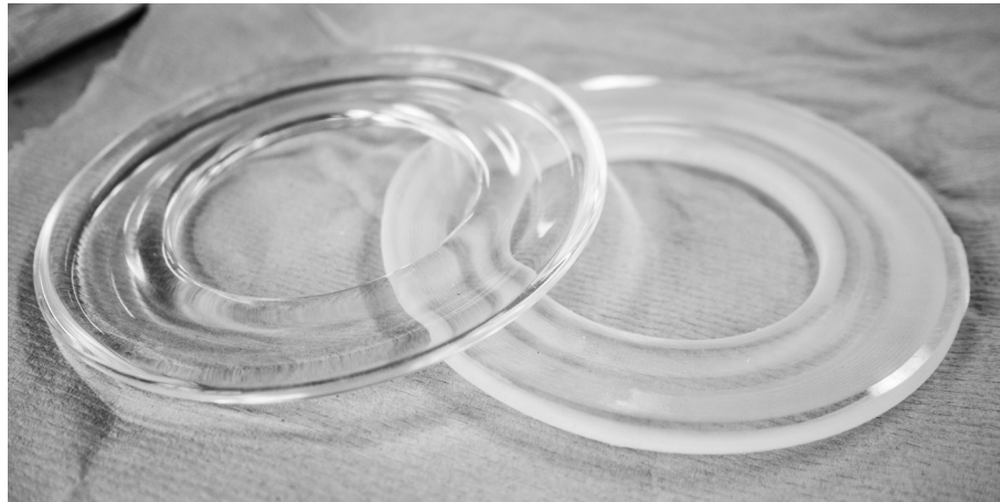
the acrylic top was first cnc-machined, then hand-polished
