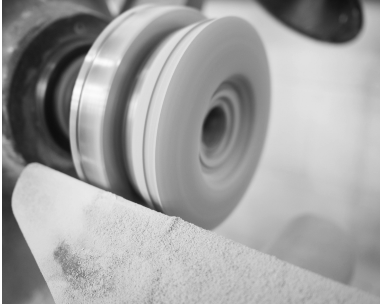
turning high-density foam on a lathe
