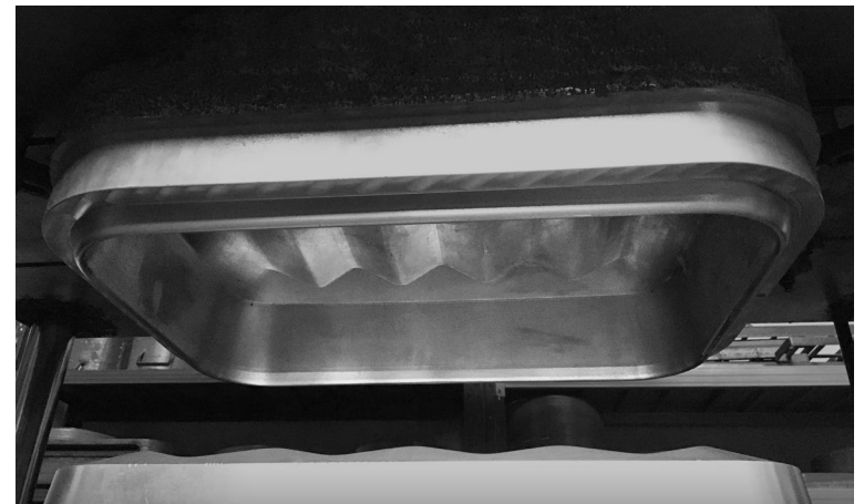
the cast steel mold to produce the bins
